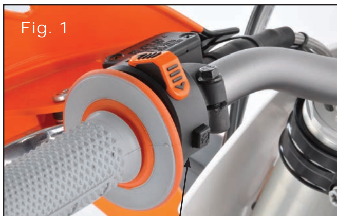
TRAIL TECH IGNITION MAP SWITCH INSTALLED
