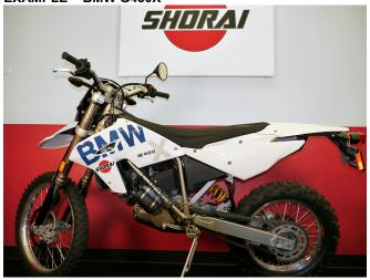
The factory-installed battery in the BMW G450X is Yuasa lead-acid YTZ7S. Our standard recommendation for Shorai Lithium-Iron is LFX09A2-BS12. The LFX09A2 weighs 3.31 lbs less than the original YTZ7S (or 1.5Kg, ~73% lighter), has less than 1/6 the self-discharge rate, and cranks the engine 20% faster!
