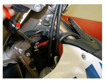
Max torque for the terminal screws is 4.5kg/cm (60 oz/inch). Do not over-tighten. We recommend the use of a #3 (big!) Phillips screwdriver, as this allows you to apply downward pressure on the terminal screw. That helps the threads catch, and reduces torque on the terminals. Note that the terminals are not anchored at back, and may twist slightly during install. If so, performance is not affected.
