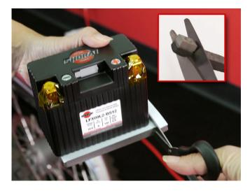
In this example, we only needed to shim the height. Do the same if the original battery is significantly larger in width or depth, and trim the selected spacers to fit with scissors.
