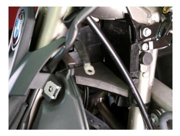
The LFX batteries can bolt cable eyelets to either the top or front sides of the terminals. **Be sure to Install the POSITIVE terminal cable first**, then Negative, to avoid short circuits.
