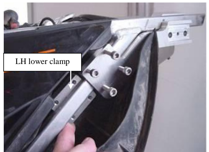
Figure 4: Install of LH lower clamp
