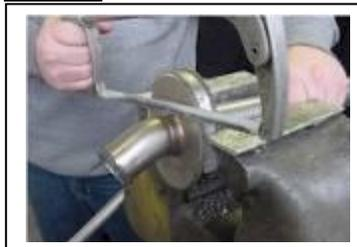
The perforated inner core will now be separated from the steel end cap. **FIGURE 5**
