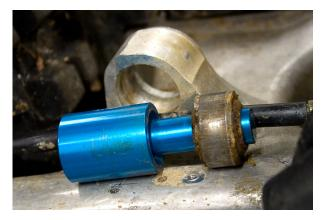
4. Place the bearing extractor on the handle and insert through the center of the heim joint. Drive the bearing out using a mallet.
