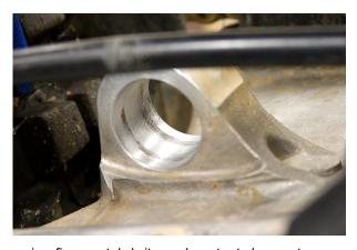
5. Carefully clean the inside of the swing arm bearing surface using fine scotch-brite and contact cleaner to remove any burrs or corrosion.
