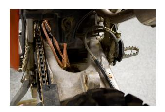
1. Remove shock, inner fender mud flap, and brake line clip.
