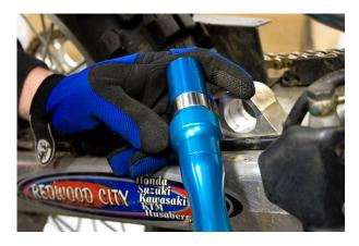
6. Place the new bearing onto the bearing extractor and then into the installation adapter with the recess facing the bearing. Then insert handle into Installation adapter as shown.
