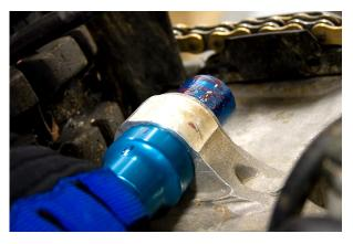
7. Place a light coat of grease or assembly lube on both the bearing and the bearing extractor to prevent damage during the installation. Rotate the flat portion of the installation adapter so it is aligned with the flat on the shock mount boss. Using a mallet, drive the bearing into the boss until it is fully seated against the installation adapter.
