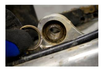
3. Remove right heim joint seal using a seal puller or a flat blade screw driver. When removing the seal be careful not to scratch the inside of the shock mount boss.
