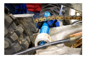
8. Using the extraction adapter, carefully install the new seals until they are flush with the sides of the shock mount boss.
