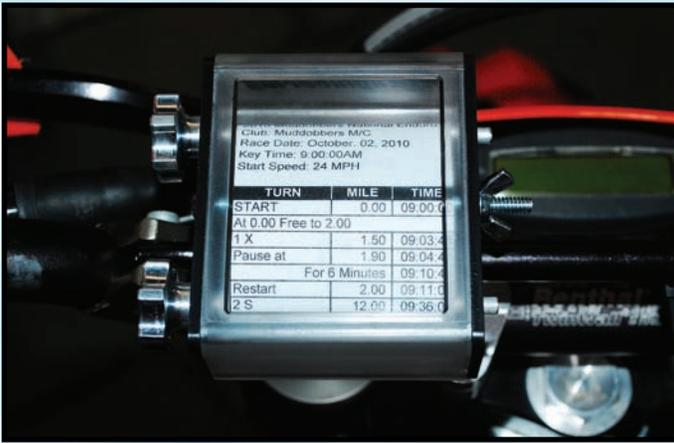
**1** Installation on bikes with Fat Bars or bikes that do not have a crossbar. Place Roll Chart Holder over left side of handle bars, the bar will fit into the cradle of the rubber hose and clamp. (Fig 1)
