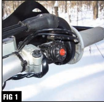
**2** Remove the backing from the backside of the heat pads. Stick one directly to the left side of the handlebar so that the wires are on the top side of the handlebar. Stick the other one to the throttle tube so that the wires are on the top side of the throttle tube.
